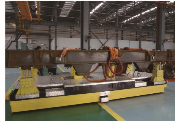
武汉大功率现场 AGVs applied in high power locomotive maintenance Wuhan base
