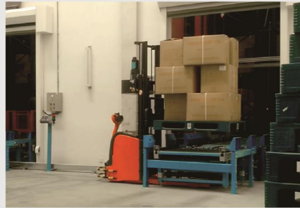
天津力生制药现场 AGVs applied in Tianjin Lisheng Pharmaceutical Co.,Ltd.
