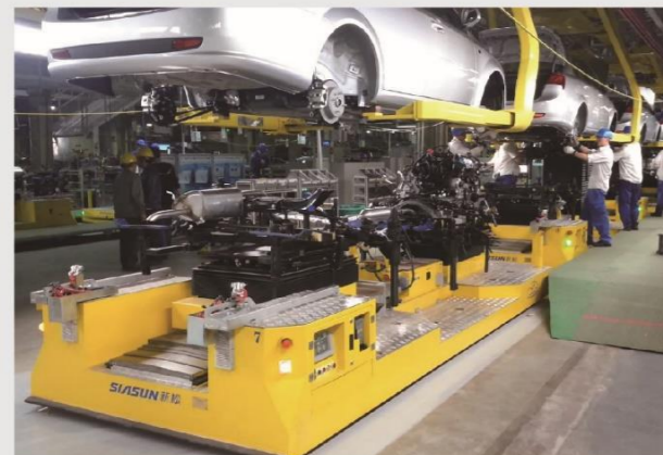
通用现场 Inductive Power Transfer AGVs applied in GM
