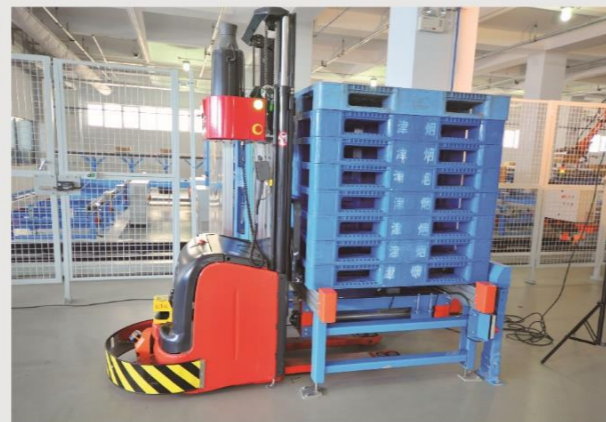
天津烟厂现场 AGVs applied in Shanghai Tobacco Group Co., LTD. Tianjin Factory.
