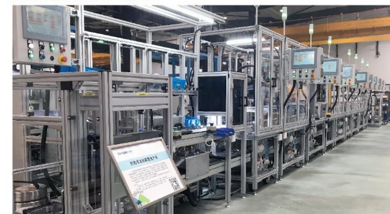
喷嘴装配线 Fuel Injector Assembly Line
