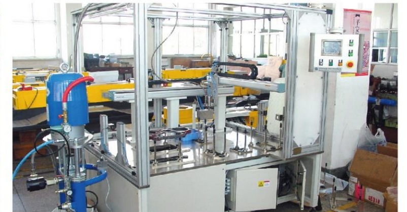
柴油发动机涂胶机 Seal system for diesel engine
