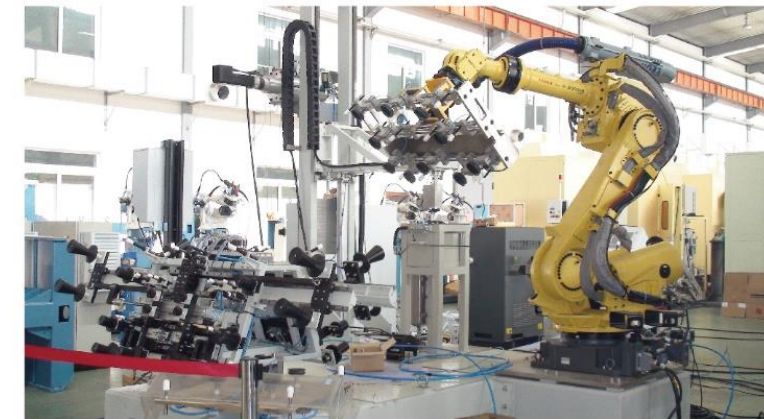
风挡涂胶 Windshield sealing robot
