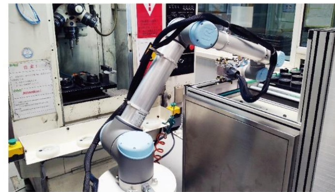
斜盘数字化加工生产线 | Inclined disk digital processing line
